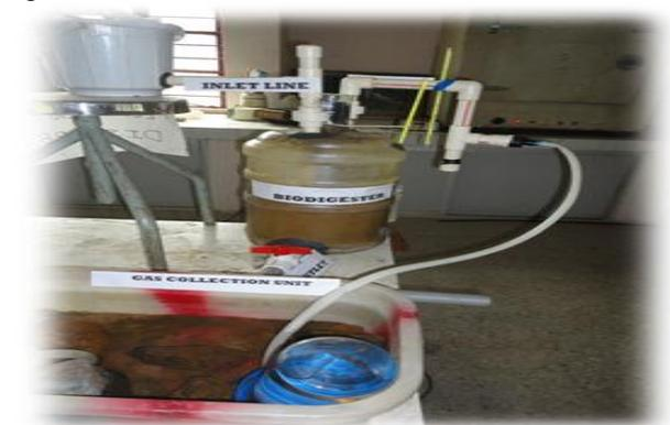
**Figure 1. Set up of the fittings of the digester and operational digester**
